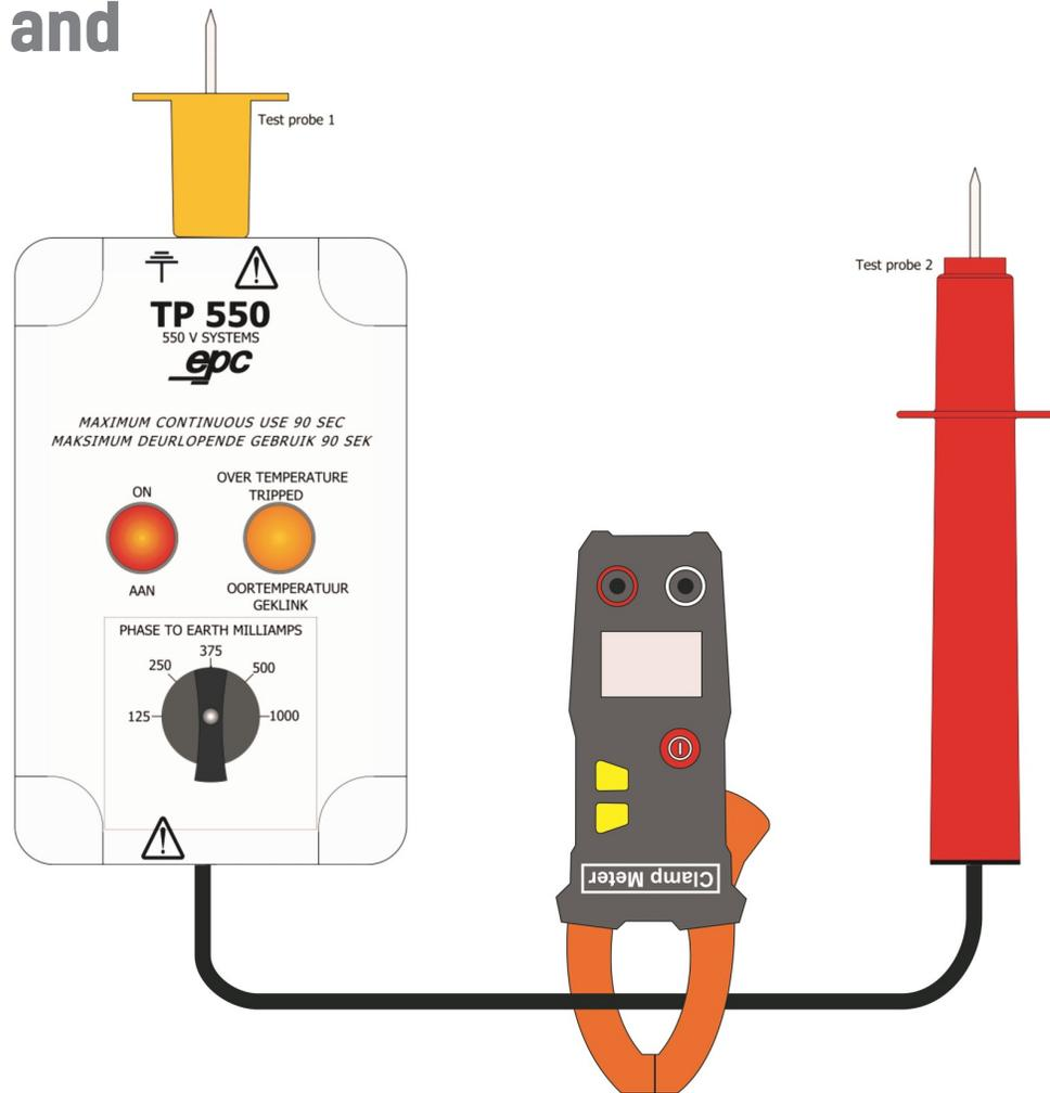
Two large diameter neon lamps, one for indicating when power is present on the test probes and one for when the thermostat has disconnected the internal circuit.
