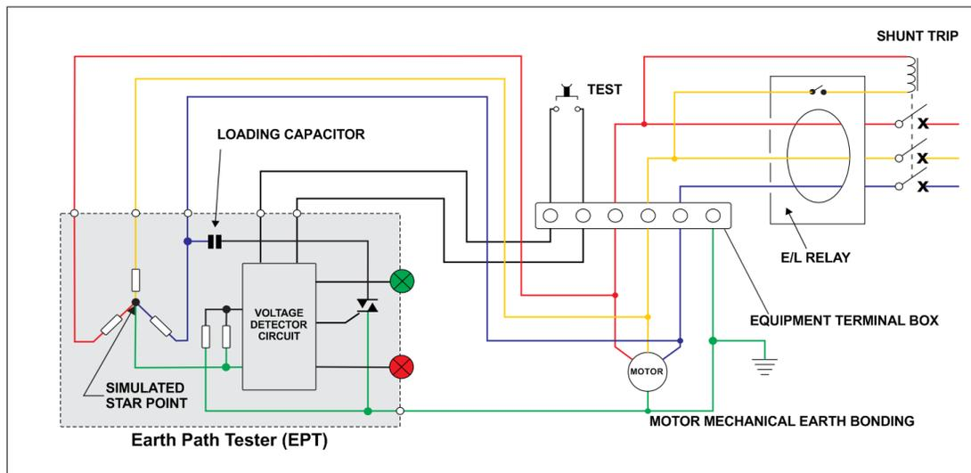
The Earth Path Tester forms a permanent maintenance free installation into equipment to be monitored.
